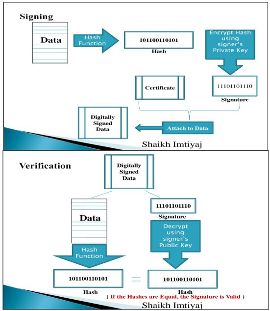
Figure.3- DSC working process
