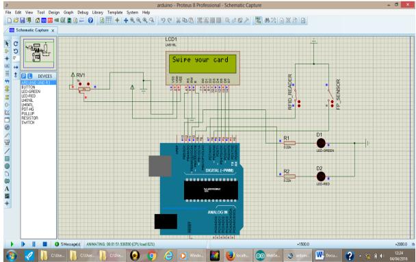
Fig. 4.2 Simulation prompting student to swipe RFID card
