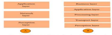
Figure 1: Architecture of IoT (A: three layers) (B: five layers).
