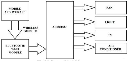
Fig 3.1 System Block Diagram
