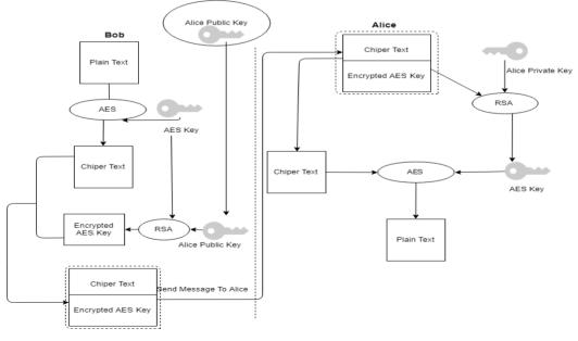
Fig.4.1 RSA 4096 Simple working process:-
