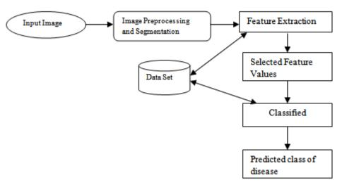
Fig 2: Basic Steps in Image processing to detect plant disease
