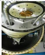
Figure 3.Pelletron generator with conducting links.
