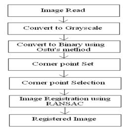
Figure 1.Block Diagram for Our Proposed Method
