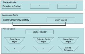
Figure 2: Two-level cache architecture
