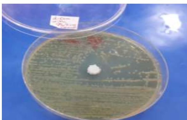
Fig. 4: Show the susceptibility (inhibition growth) of Staphylococcus aureus to the synthesis ZnO/NPs dental composite in 7% concentration prepared from this inorganic agent.
