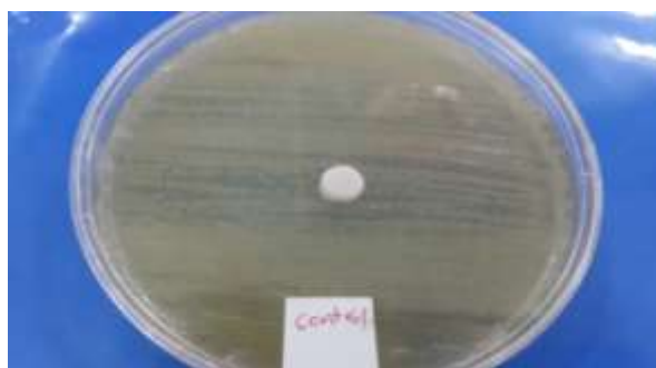
Fig. 2: Show no effect of the control (dental composite without the addition of ZnO/NPs) on the bacterial growth.
