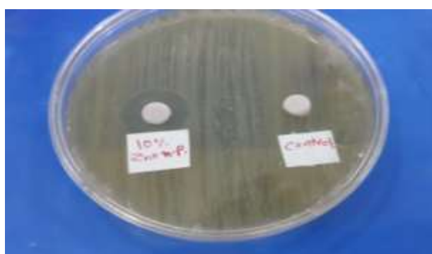
Fig. 3: Show the differences between the effect of control (dental composite resin without ZnO/NPs) and dental composite resin with addition of 10% ZnO/NPs ; (A) no inhibition growth of Klebsiella.spp (unsusceptible) to control , (B) inhibition growth of Klebsiella.spp (susceptible) to synthesis ZnO/NPs dental composite.
