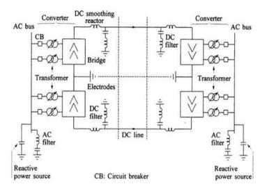
Fig. main components of HVDC system
