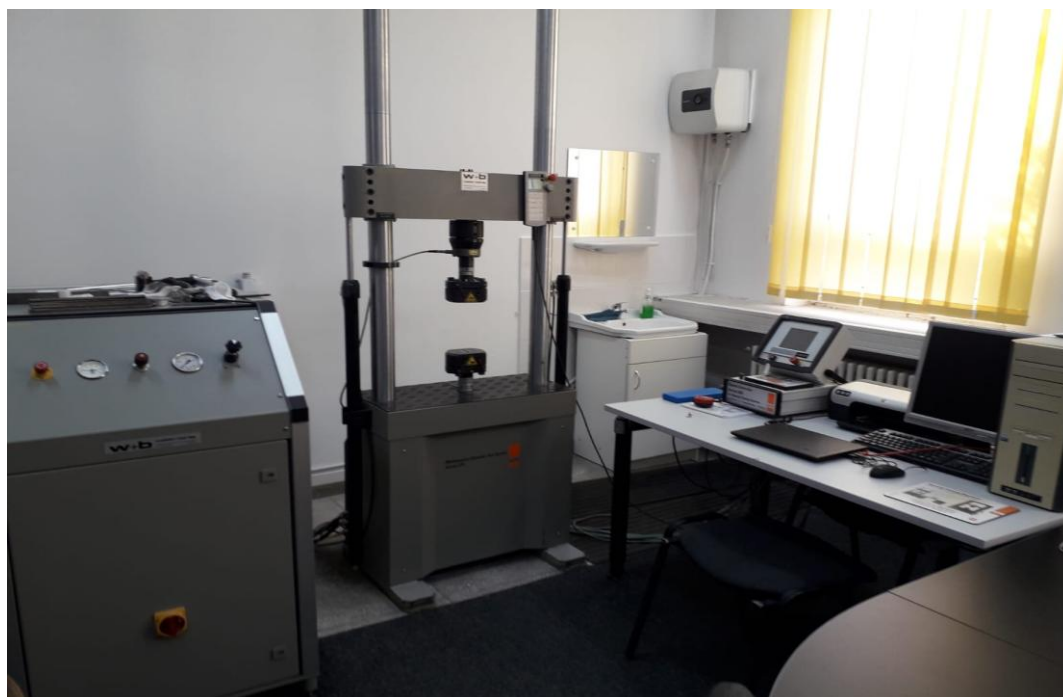
Fig. 1 Walter+bai ag 50 kN Multipurpose Servohydraulic Universal Testing Machine
