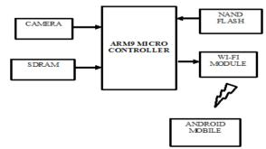
Figure: hardware implementation block diagram.
