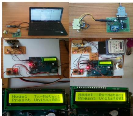
Figure 8 Designed Meter reading system prototype
