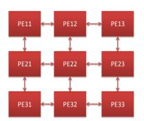
The network of processing elements consists of nine PEs and all are internally connected to each other.PE11 is connected to PE12 and PE21, PE12 is connected to PE11, PE13 and PE22, PE13 is connected to PE12 and PE23.Similarly other PEs are connected to its neighbour PEs. The PE22 is connected to four processing elements those are PE12, PE21, PE23 and PE32.
