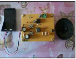
a) Transmitter circuit b) Receiver circuit Fig. 5 : The constructed prototype of the transmitter and receiver
