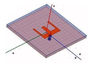
Figure 1: Design of E shaped patch antenna
