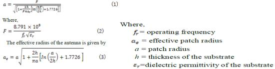
The circular microstrip antenna designed at operating frequency 2.45 GHz, having FR4 substrate with height of 1.59
