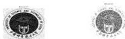
Figure 11. Extracted watermarks after JPEG compression of watermarked baboon with ratio 1.7 (left) and 2.3 (right)
