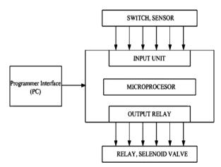
Fig 2.4. PLC (Programmable Logic Controller)
