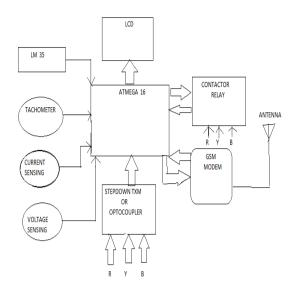
Fig 1.1 Block diagram of required system
