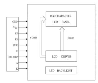
Fig 2.5: Block diagram of LCD
