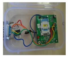
Fig 2.3. GSM Module
