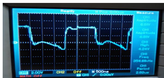
Figure12: Gate drive voltage with external frequency synchronization
