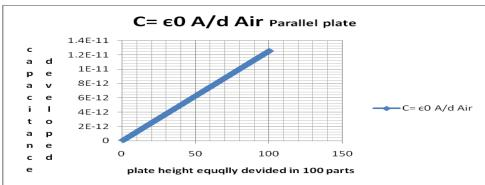
Fig.4 capacitance development in parallel plates-air
