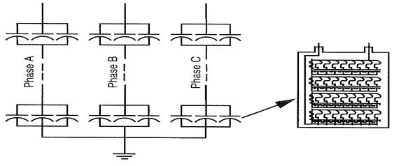
Fig.1-capacitor banks in industry having puncturing of electrode problem
