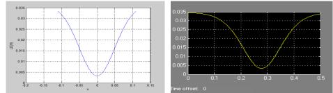
Figure (9.a, 9. b) Variation of the inductance of coil without iron nucleus  $L_0$  in function of the displacement and time.
