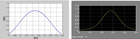
Figure (8.a, 8. b) Variation of the inductance of the nucleus L<sub>f</sub> in function of time and displacement.
