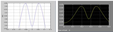
Figure (11.a, 11. b). Variation of the mutual M in function of the displacement and the time
