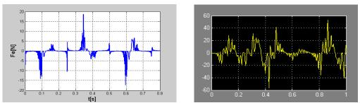
Figure (12.a, 12. b) variation of the magnetic force in function of the displacement and the time
