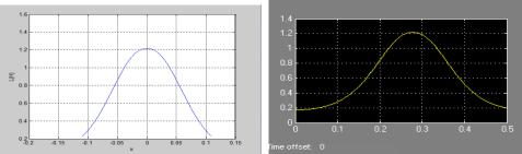
Figure (10.a, 10. b) Variation of the total inductance L in function of the displacement and the time
