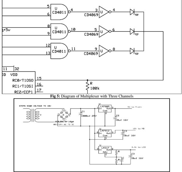
Fig 6: Circuit Diagram of the Power Supply Unit
