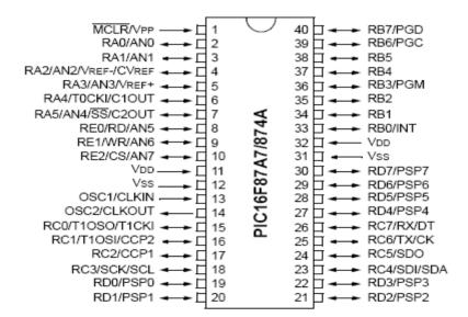
Fig 4: Pin Diagram of the Microcontroller
