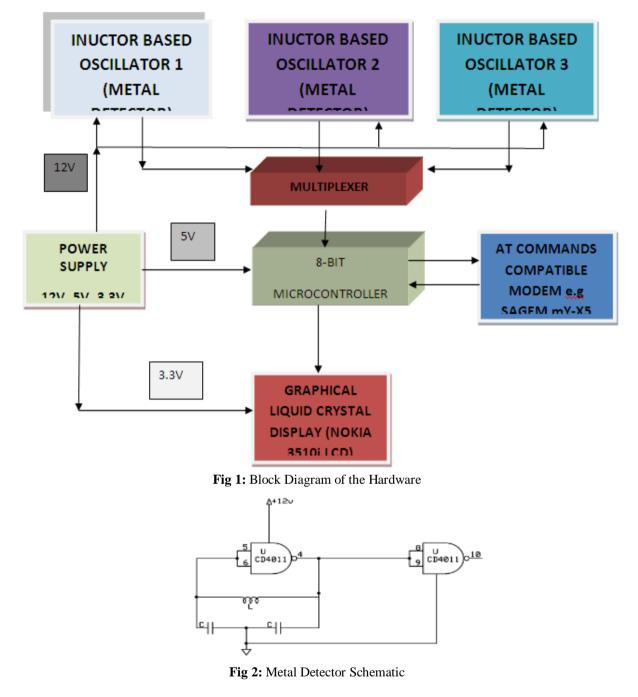
Capacitor, C= 10nF, Number of turns, N=14, Diameter of the coil, D=22cm Radius of the coil,  $r = \frac{D}{2} = 11$ cm, Length of the coil, l=7.4cm = 0.074m The cross-sectional area of the coil, which is circular, is given by,  $A = \pi r^2$ ,  $A = \pi \times 11^2 = 380.13$  cm<sup>2</sup>=0.038013m<sup>2</sup> In accordance with electromagnetic theory, the inductance of an inductor is given by,  $L = \frac{N^2 \mu A}{l}$ . Where  $\mu$  is the permeability of the coil
