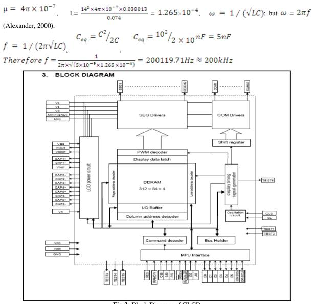
Fig 3: Block Diagram of GLCD
