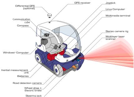
Fig. 2 sensors and actuators of the electric vehicle Cycab
