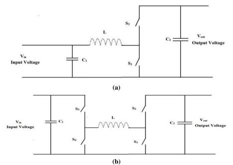
Fig.2. Topologies of (a) Half bridge converter, (b) Cascade converter [6].
