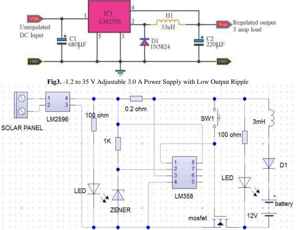
Fig.4: Complete diagram of cost efficient solar PV charge controller
