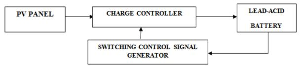
Fig.2: Simplified Hardware Block Diagram of a Solar Charging Station
