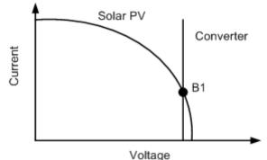
**Fig.1:** Characteristics of PV voltage controller
