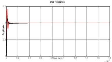
Fig 5. Unit step response of the monotonic compensation (dashed line) and the non-monotonic compensation (solid line).
