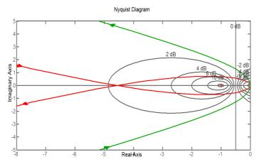
Fig 4. Nyquist plots for the monotonic compensation (dashed line) and the non-monotonic compensation (solid line).
