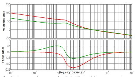
Fig 3. Bode plots for the monotonic compensation (dashed line) and the non-monotonic compensation (solid line)
