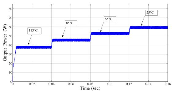
Fig. 8. Output Power of Boost Converter at different temperature values
