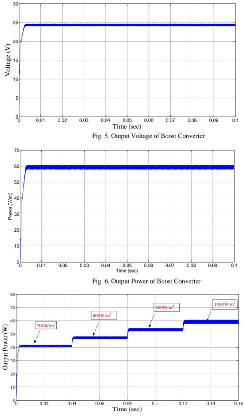
Fig. 7. Output Power of Boost Converter at different insolation values
