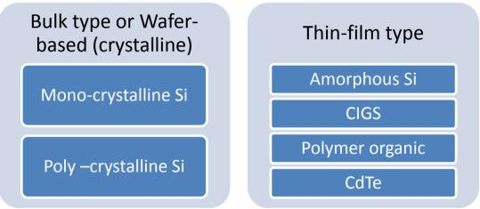
Fig. 2 classification of solar panels
