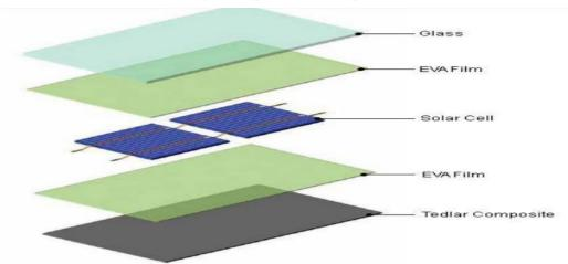
Fig.1. Components of solar panel
