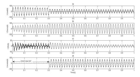
Fig.5. (a) Load Current. (b)Source Current. (c)Current from Wind turbine Induction Generator.(d) Inverter Injected Current
