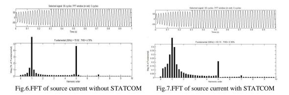
Power quality improvement (i.e.) harmonic distortion reduction is observed at PCC when STATCOM is on as shown in Fig 7. THD is reduced considerably to 0.36% which is within norms prescribed by grid code.
