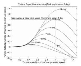
Fig.2.PowerCharacteristics of Wind Turbine
