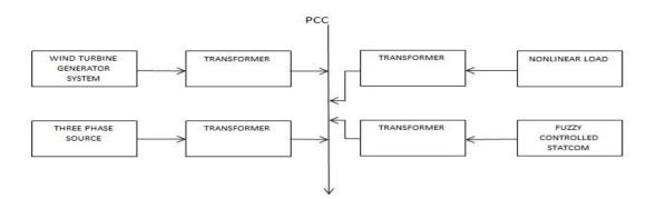
Fig.1.Simulated windfarm Topology
