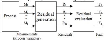
Fig. 3: The general structure of a diagnostic system
