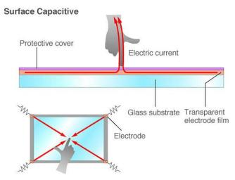
Fig.14. Layered structure of touch screen
