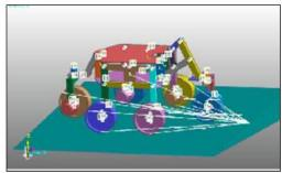
Fig.7. Shrimp rover model in RecurDyn
