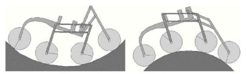
Fig.6. Structure on concave and convex ground
