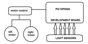
Figure 3: block diagram of the follower robot [2]
