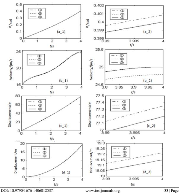
Figure 5. Model comparison for lane changing:  $(a_1)$  Angular displacement;  $(a_2)$  Partial enlargement of  $(a_1)$ ;  $(b_1)$  Velocity of vehicle;  $(b_2)$  Partial enlargement of  $(b_1)$ ;  $(c_1)$  Displacement along X-axis;  $(c_2)$  Partial enlargement of  $(c_1)$ ;  $(d_1)$  Displacement along Y-axis;  $(d_2)$  Partial enlargement of  $(d_1)$
