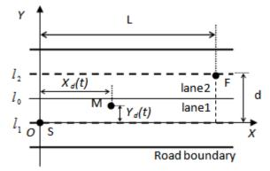
Figure 1. Schematic diagram of trajectory planning for lane changing on straight road
