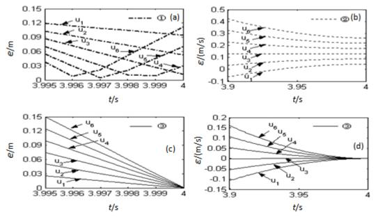
Figure 9. Simulation result with different values of velocity at end time: (a) Position deviation using method(1); (b) Position deviation using method(2); (c) Position deviation using method(3); (d) Velocity deviation using method(3)
