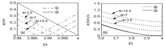
Figure 7. Simulation results with different lane spacing: (a) Position deviation; (b) Velocity deviation
