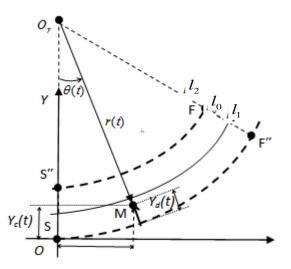
Figure 3. Schematic diagram of trajectory planning for lane changing on circular road
