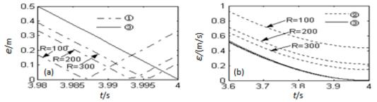
Figure 6. Simulation result with different radii of road: (a) Position deviation; (b) Velocity deviation
