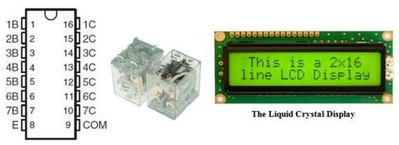
Fig 4. The ULN2003A Pinout, 12V Relay and LCD (source: futurelec.com)
