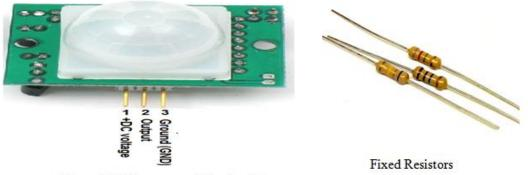
Figure 3: PIR sensor and fixed resistors.
