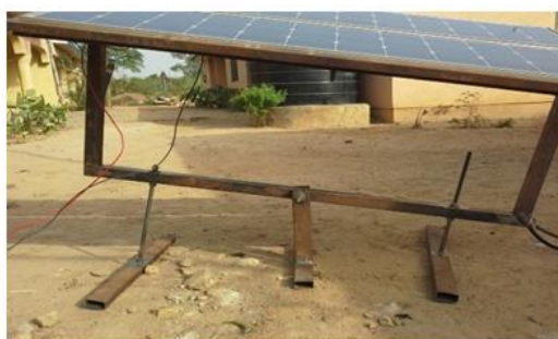
Figure 1.6: Base frame spring support
