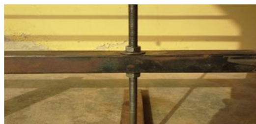
Figure 1.4: Joint middle support (Pie shaped base and U-shaped cross bar)
