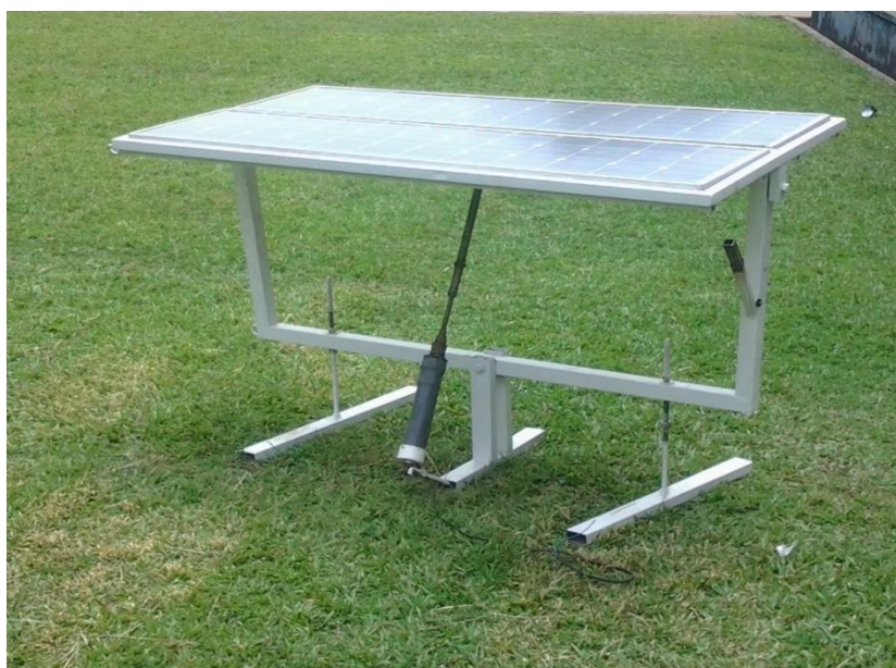
Figure 1.7: Single Axis Solar tracker
