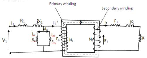
Fig. 1: Per-phase equivalent circuit of a transformer on load.
