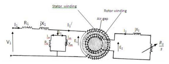
Fig 2: Per-phase equivalent circuit of an induction motor
