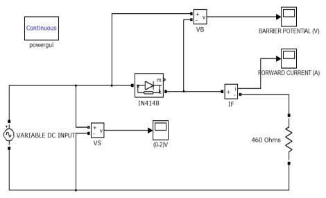
Fig 1.a.Forward bias circuit arrangement
