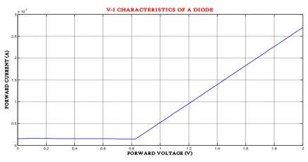
Fig 1.e.Forward voltage and current characteristics of diode
