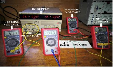
Fig 3.b.Forward bias experiment with two dc supply
