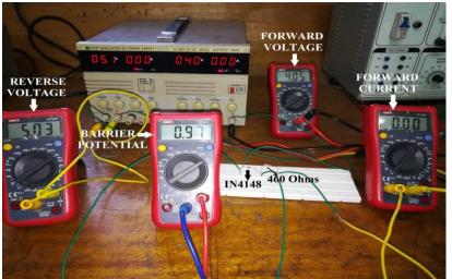
Fig 4.b.Reverse bias experiment with two dc supply
