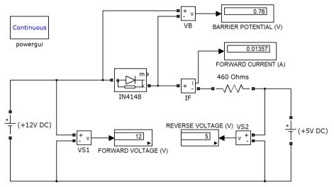
Fig 3.a Forward bias circuit arrangement with two dc supply
