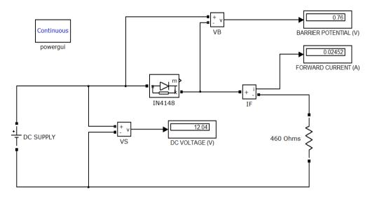
Fig 2.a Forward bias with fixed dc input voltage
