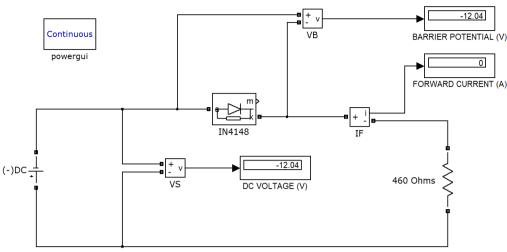
Fig 2.c.Circuit arrangement of reverse bias
