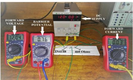
Fig 2.b.Forward biasexperimental setup with fixed dc input voltage
