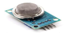
Fig.5. MQ-6 gas sensor
