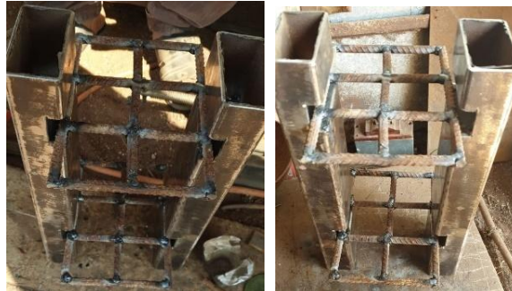
(Figure2.1 TMT Bars Structure with MS Pipe)
