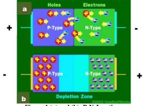
Figure 1 (a) and (b): P-N Junction
