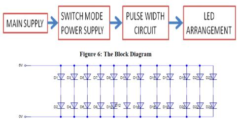
Figure 7: LED Arraignment
