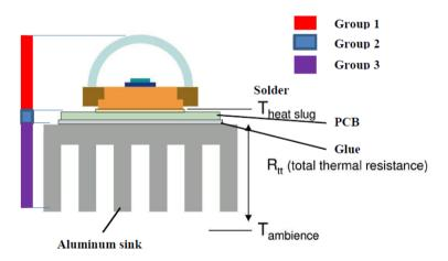
Figure 3: Schematic diagram of LED bulb structure
