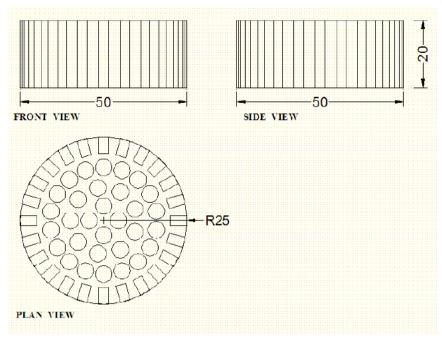
Figure 4: Orthographic view of NASENI-ELDI (Pin-Trapezium Hybrid Heat Sink) LED Bulb
