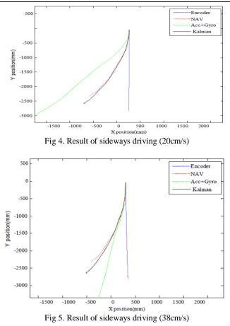
In the result (--) which uses only the encoder, the driving result of the AGV seems like moving straight. But if you see the result (:) using NAV200, we can verify that the AGV don't moved straight by the slip. In case of using accelerometer and gyro, the result (-.) has high errors by the double integral of accelerometer. However, the result (-) of the proposed method is similar to the result of NAV200. Table 2 shows each of the experiments.
