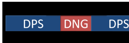
Figure 1: Cross section of Planar Antenna on DPS-DNG-DPS Composite
