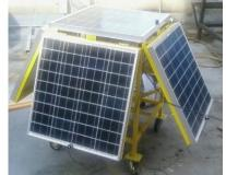
Figure 3: Orientation of PV modules at 4 different slopes [9].
