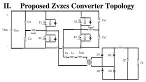
Fig 2.Proposed ZVZCS full-bridge converter
