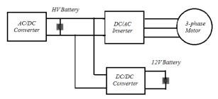
Fig.2. Block Diagram Of EV Power Conditioning System
