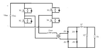
Fig.1. Conventional full-bridge converter`
