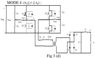
Fig.3 (d) Shows the active circuit during this mode. In this interval the output capacitor of  $S_3$  is discharging from and that of  $S_4$  is charging up to  $V_{dc}$ . This mode ends when the  $S_3$  output capacitor got completely discharged and  $S_4$  output capacitor got charged to  $V_{dc}$ . At the end of the mode 4,  $V_{AB}(t_4) = 0$  [1].
