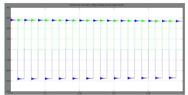
Fig. 5.Transformer secondary voltage, voltage across diode of Conventional full bridge converter
