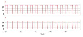
Fig 5. Control signal for switches S1 and S2
