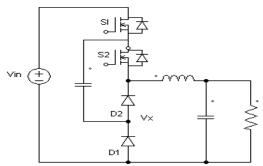
Fig. 1 Flying Capacitor Three level buck converter
