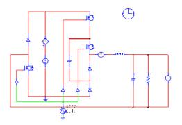
Fig. 4. Circuit layout of Modified Flying Capacitor three level buck converter in PSIM
