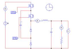
Fig. 3. Circuit layout of Flying Capacitor three level buck converterin PSIM
