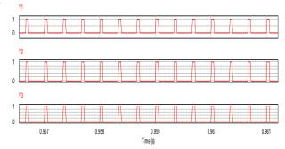
Fig. 9. Control signals for auxiliary switch, switch S1 and Switch S2
