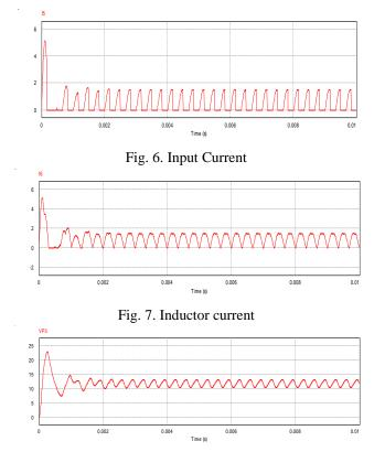
Fig. 8. Output of three level buck converter
