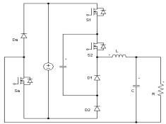
Fig. 2 Modified Flying Capacitor converter topology
