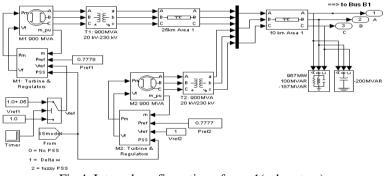
Fig 4. Internal configuration of area 1(subsystem)
