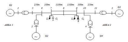
Fig 2. One line diagram of two-area four-machine system
