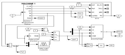
Fig 5. Internal configuration of Turbine and regulator (subsystem)
