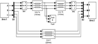
Fig 3. Simulink model of two area four machine system
