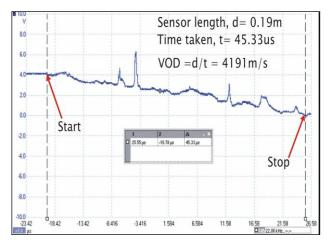
Fig.2 Voltage-Time (µs) graph to calculate VOD
