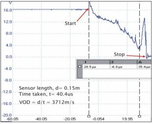
Fig..4 Voltage-Time (µs) graph to calculate VOD
