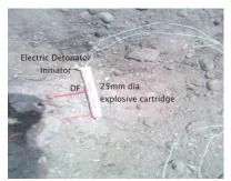
Fig. 2 D'autriche method in field Fig. 2 D'autriche method in field
