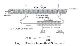
This method of VOD measurement is suitable for unconfined measurements only. See Fig. 2 below.
