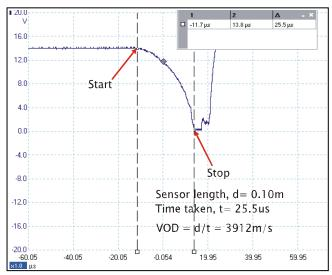
Fig.5 VOD record of SMD sensor in cartridge emulsion explosive 25mm paper tube type.
