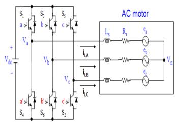
Fig.3: three-phase voltage source pwm Inverter
