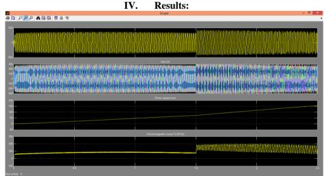
Fig shows the simulated waveforms for the output voltage, current (Iabc), rotor speed, electromagnetic torque v/s time. We observe a step speed reference change at 1.5s in waveforms.
