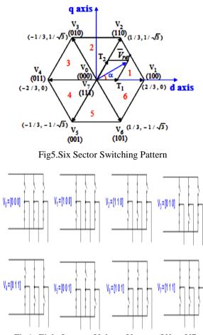
Fig6. Eight Inverter Voltage Vectors (V0 to V7
